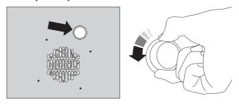
Taking care to protect your fingers in case the bulb should shatter, unscrew the old bulb.
